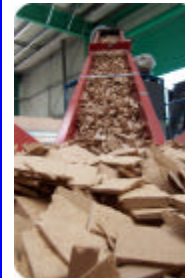
Waste MDF prepared as gasifier fuel
